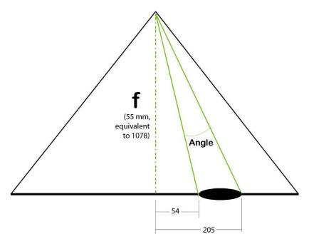
Figure 16- Angle of view within camera.
